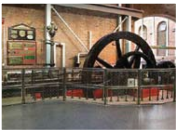
Horizontal condensing engine, Museum of Science & Industry
